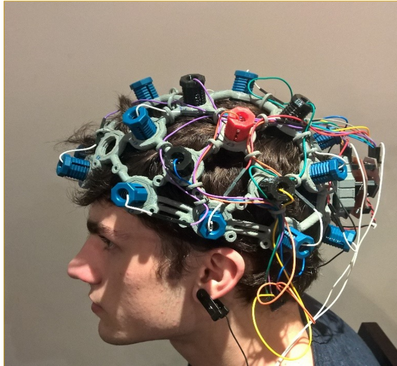
Fig. 3: An OpenBCI 3D printed EEG cap with integrated HD-tDCS. The blue electrodes are EEG, the red electrode is the anode (tDCS), and the black electrodes are the cathodes (tDCS)
